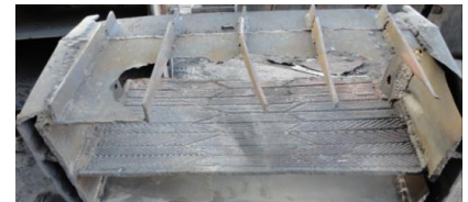
Burner tip plates after 15months of field trials showing intact laser clad plate and worn out uncoated plate at top
